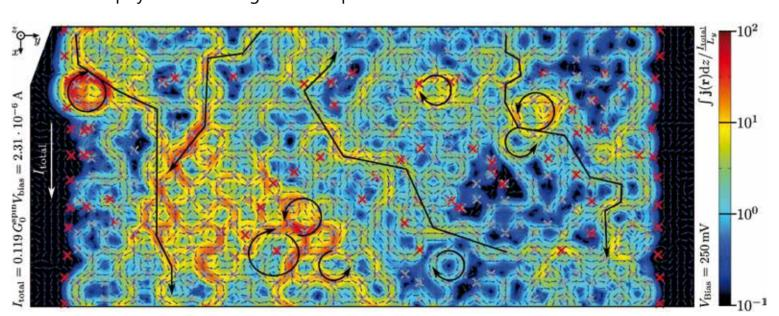
Above: Distribution of local currents flowing through a (armchair) graphene ribbon. It is 40 carbon atoms wide and has been functionalized with 20% hydrogen coverage. A net current is flowing from top to bottom. As indicated by the arrows, on a local scale the average current cannot be resolved; due to the presence of eddies in large areas of the sample the typical local current exceeds the average current by factor of five.
